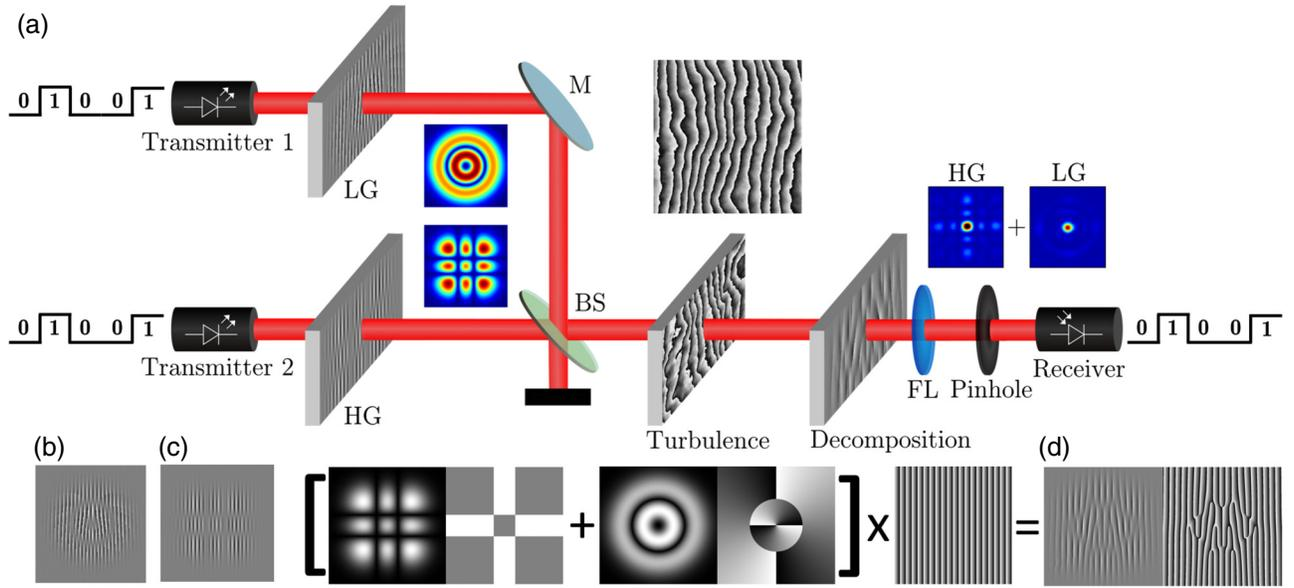
FIG. 3. Experimental setup showing two transmitters and a single receiver for transmit diversity with example turbulence as an inset (a). The holograms along the bottom are for (b) generating an  $LG_{\ell=2}^{p=1}$  beam, (c) generating an  $HG_{n=2}^{m=2}$  beam, and (d) superposition of the generated LG and HG beams to a single detector. The flat gray areas on the holograms is due to complex amplitude modulation.
