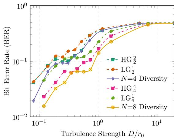
FIG. 4. Bit error rate of modes with order  $N = 4$  and 8, where  $D = 1.4$  and 1.98 mm, respectively, with varying turbulence strength showing a clear improvement for the diversity cases. Larger modes are expected to experience lower turbulence in comparison to smaller modes.
