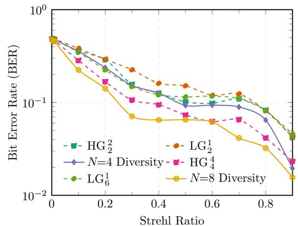
FIG. 5. Bit error rate of modes with order  $N = 4$  and 8, with varying turbulence strength in terms of the Strehl ratio for  $D = 1.4$  mm. The diversity case is typically better than the nondiversity cases with significant gains in weaker turbulence.
