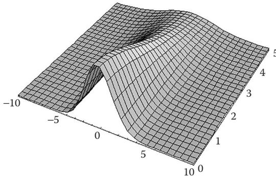
FIGURE 7.7 Intensity changes in a Gaussian beam ( $\omega_0 = 3 \text{ mm}$ ,  $M^2 = 1$ ,  $\lambda = 10.6 \text{ }\mu\text{m}$ ) over 5 m.
