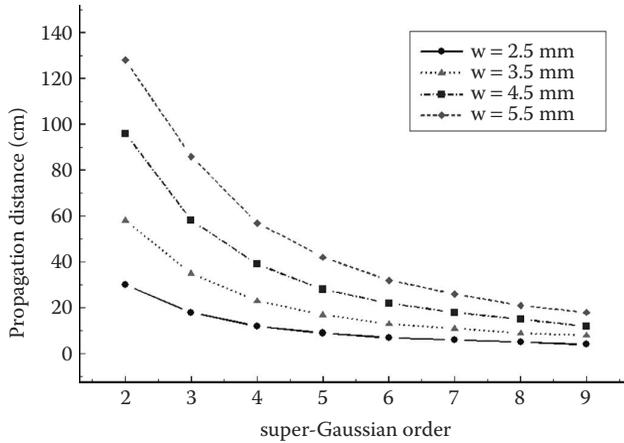
**FIGURE 7.6** Maximum propagation distance as a function of super-Gaussian order and starting beam size ( $w$ ), for a 10% rms change in intensity distribution. The starting field was taken as having a flat wavefront, so that the beam size  $w$  is equivalent to the  $w_0$  of Equation 7.9.
