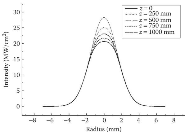
FIGURE 7.9 The Gaussian beam flattens as it propagates through the medium.
