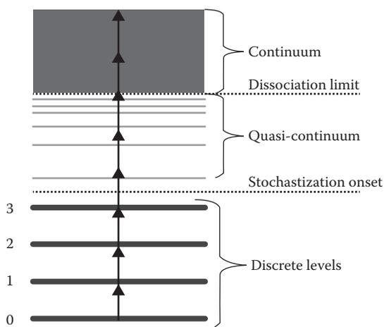
**FIGURE 7.1** A simple model of multiple-photon dissociation of a molecule by an IR laser.
