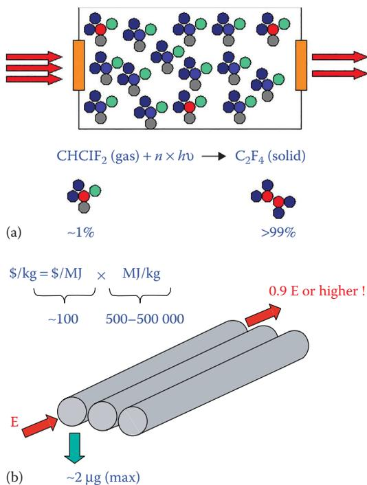
**FIGURE 7.3** (a) Energy enters a chamber with a mixture of isotopes. Molecules with one of the isotopes absorb energy, whereas the other molecules do not. After dissociation, the selected isotope is found in a different chemical compound, (b) A simple pipe version of the irradiation process, with each pipe representing the beam irradiation volume of a single pass.
