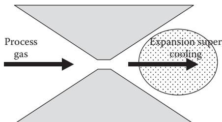
**FIGURE 7.2** A de Laval type supersonic expansion nozzle can be used to create super cooled gas. The rapid expansion creates cooled monomers, having a *clean* vibrational spectrum; this is essential for many isotope separation processes. The shaded area indicates the region where the laser beam(s) pass through. The laser beam direction is usually perpendicular to the gas flow.
