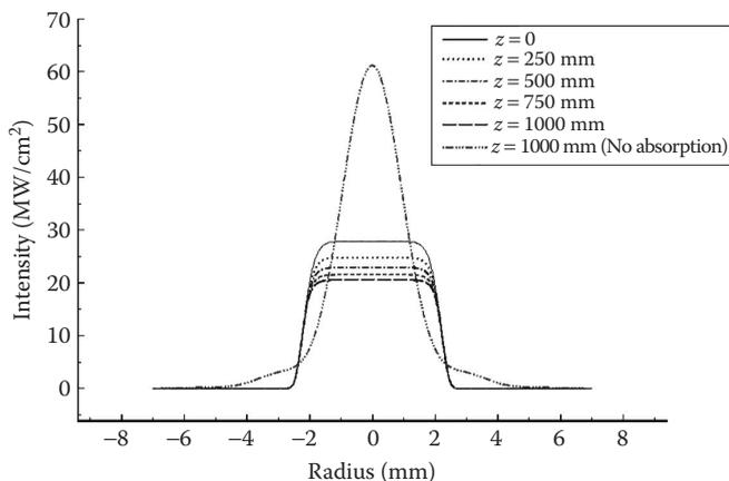
**FIGURE 7.10** The super-Gaussian beam holds its shape for longer due to the suppression of intensity spikes.
