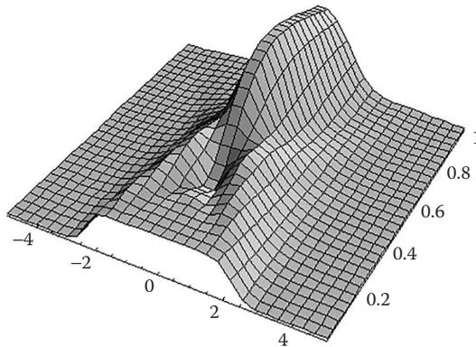
FIGURE 7.8 Intensity changes in a super-Gaussian beam ( $\omega_0 = 2.39 \text{ mm}$ ,  $p = 5$ ,  $\lambda = 10.6 \text{ }\mu\text{m}$ ) over 1 m.
