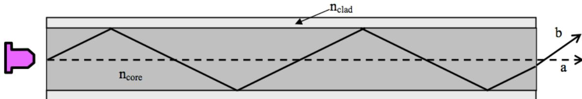
The core of the fiber has a constant index of refraction ( $n_{\text{core}}$ ) which is a little larger than the index of refraction of the cladding ( $n_{\text{clad}}$ ). Such a fiber is called a step-index multimode fiber.
