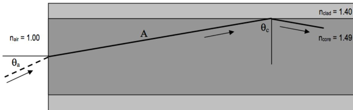
Figure 1. Cross section of a plastic fiber
