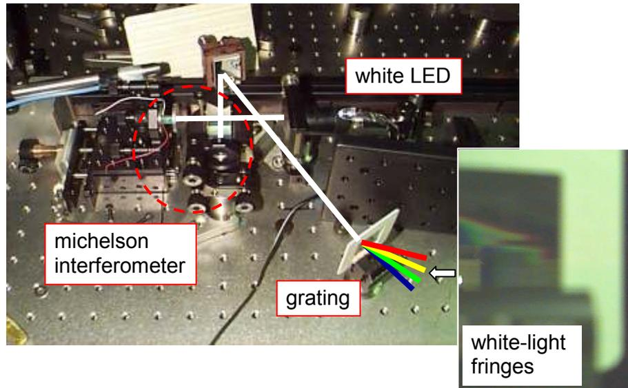
Fig. 10. Setup for observing white-light fringes “by eye.” The light from a white LED is sent to an interferometer, and then redirected to a diffraction grating. White-light fringes (i.e., a broken spectrum) is seen through the grating at the equal-arm-length position.
