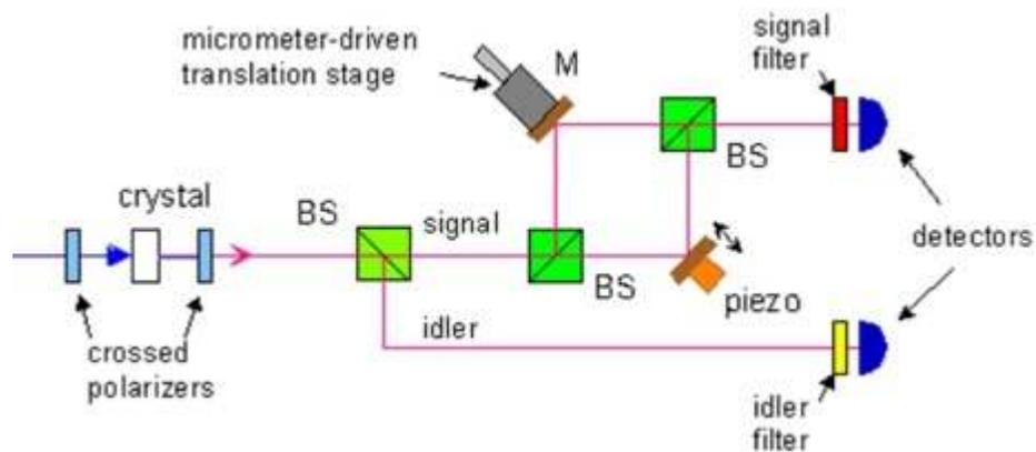
Fig. 6. Simplest layout for interference experiments.
