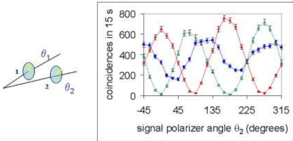
Fig. 20. Measurements of the photon correlations when the pairs are in the state given by Eq. (5). In the data sets are for  $\theta_1 = 0$  (red) with  $\theta_1 = \pi/4$  (green) and  $\theta_1 = \pi/2$  (blue).
