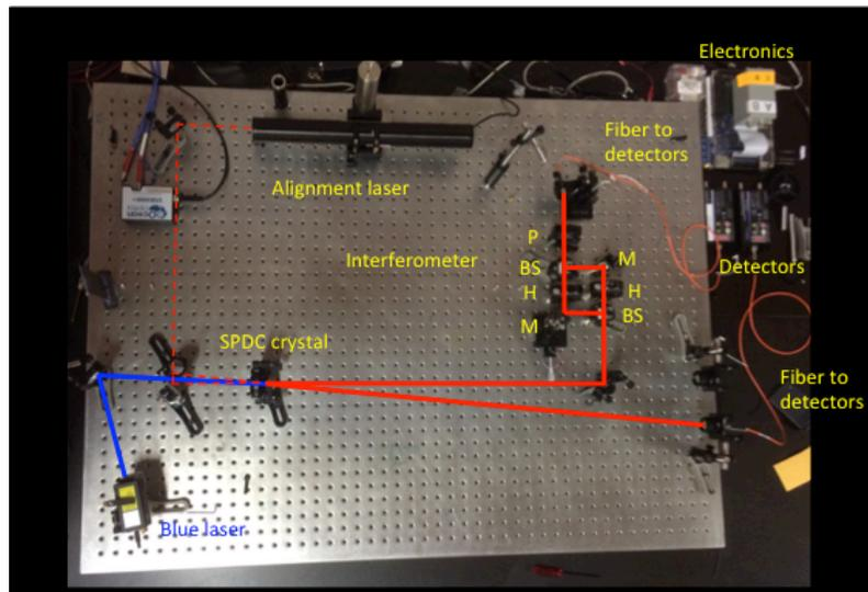
Photons go to detectors through fibers. The detectors produce electronic pulses that go to counters and a coincidence circuit. The length of one of the arms of the interferometer is scanned with a piezoelectric.
