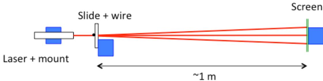
Using  $d \sin \theta = n\lambda$  find the diameter  $d$  of the wire. The (small) angle  $\theta$  is between incident direction (central maximum and  $n$ -th minimum).
