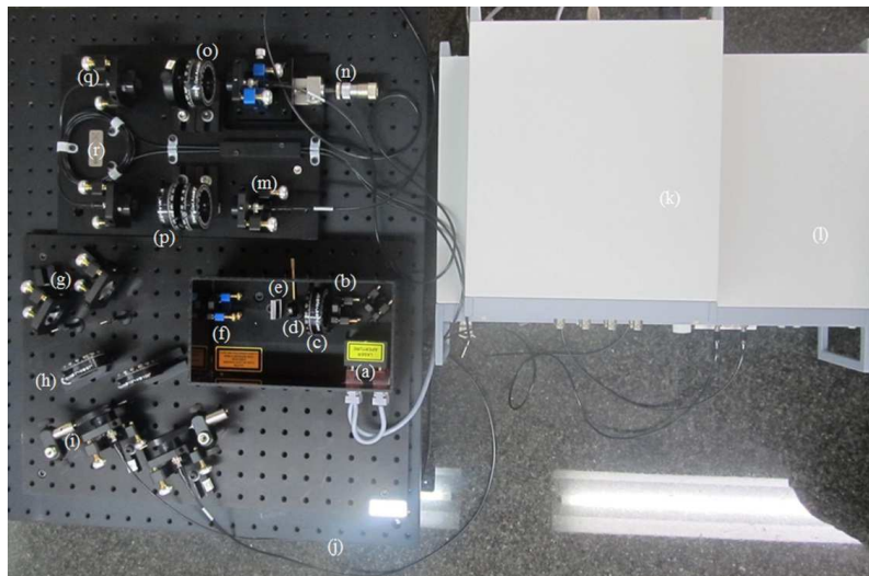
Fig.5: Optical system constructed to generate and characterize single photon pairs: (a) UV pump laser lasing at 404 nm, (b) spherical lens, (c) Half Wave Plate (HWP), (d) receiving collimators, (k) Time to digital convertor, (l) coincidence counter embedded with single photon detectors, (m) transmitting collimators, (n) manual micrometer translation stage (o) Quarter Wave Plate (QWP), (p) HWP, (q) receiving collimator and (r) is the 50: 50 polarization maintaining fiber coupler.
