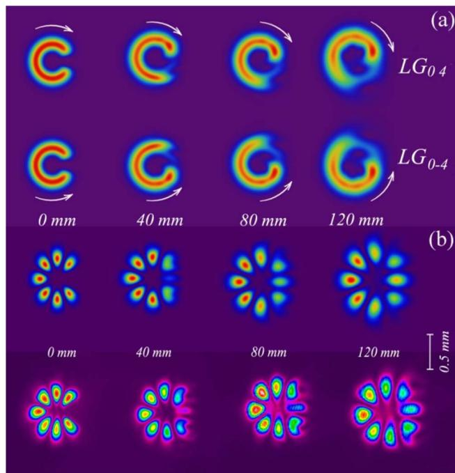
Fig. 3. (a) Simulation of the free space propagation of obstructed  $LG_{04}$  and  $LG_{0-4}$  beams. (b) Simulation and corresponding experimental verification of the reconstruction of the superposition beam ( $LG_{04}$  and  $LG_{0-4}$ ).
